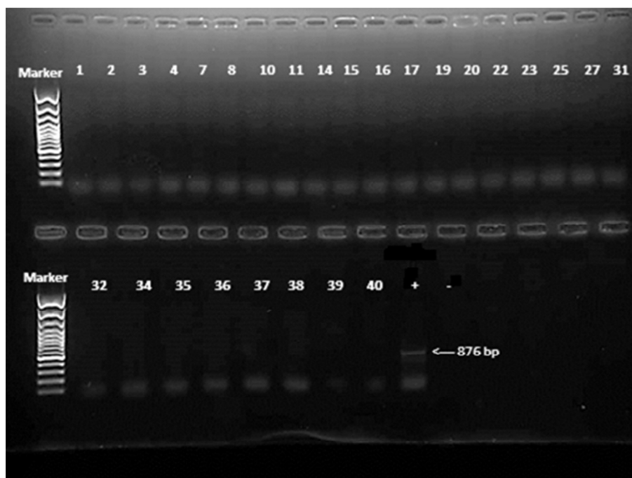
Figure 6: Agarose gel electrophoresis columns without genetic fragments of 27 Cacopsylla pruni samples (No. 1–40) from nested PCR (marker: 100 bp DNA ladder)
